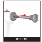
Push and hold the release button, removing the plunger shaft from the handpiece.
