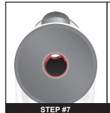
Inspect the inside of the handpiece shaft for any visible gutta percha.
